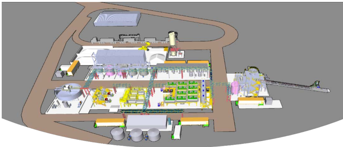
Figure 8: Proposed Modular Concentrator – Whim Creek Project
