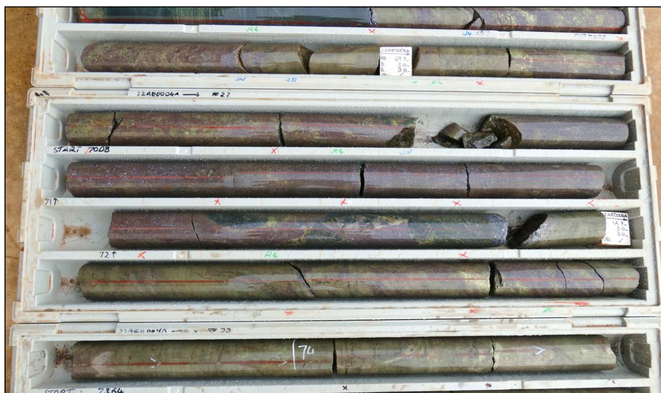
Figure 5: Massive chalcopyrite-sphalerite-pyrrhotite-pyrite mineralisation with strong disseminated galena intersected within 22AED004A.
