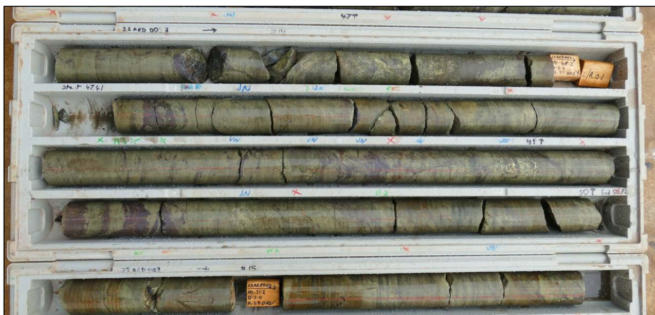
Figure 4: Massive chalcopyrite-sphalerite-pyrrhotite-pyrite mineralisation intersected within 22AED003.
