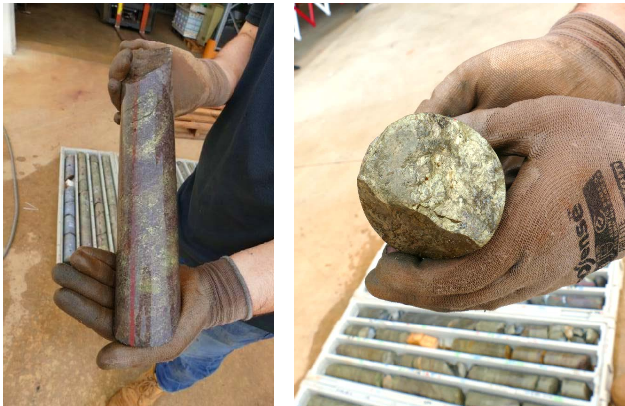
Figure 3: Massive sulphide copper-zinc mineralisation in 22AED003 and 22AED004A
