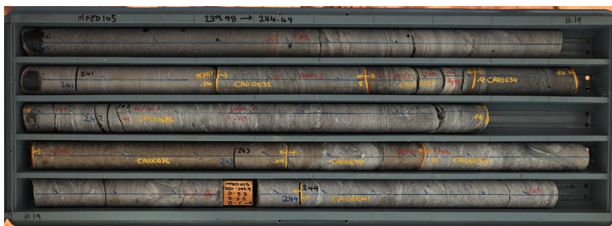
Figure 3. Core photos of mineralised section in hole MFED105
