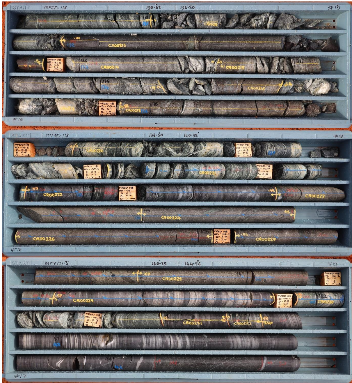
Figure 2. Core photos of mineralised section in hole MFED118
