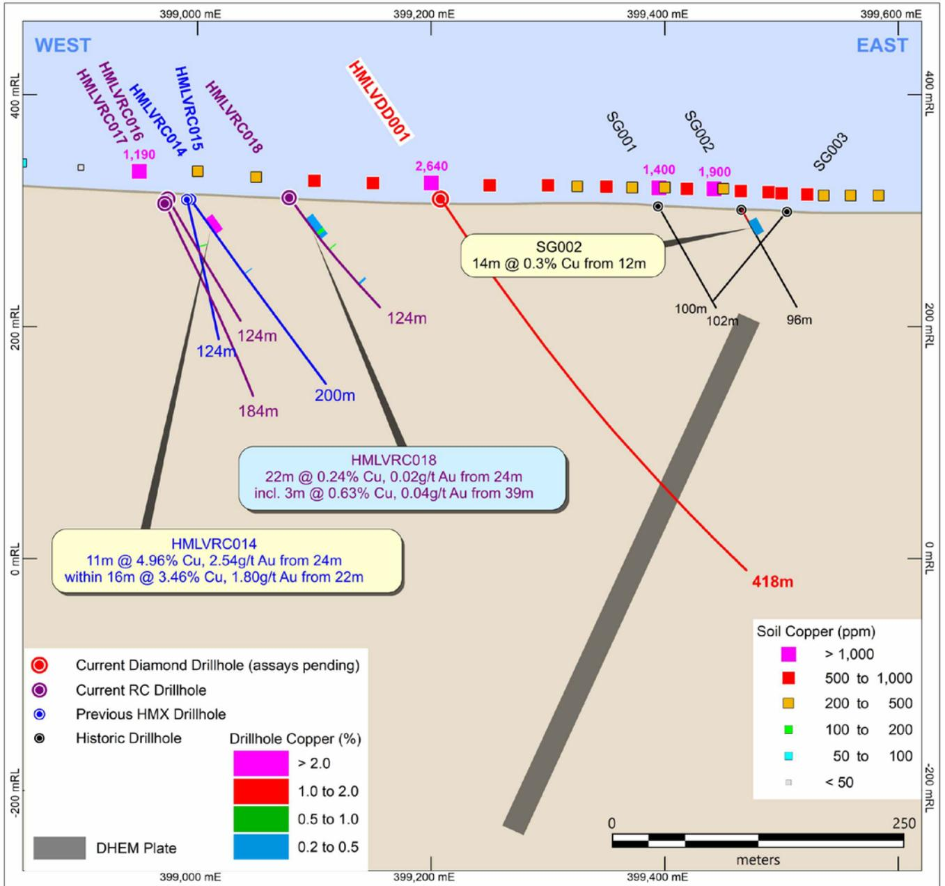
**Figure 1.** Section through HMLVDD001 showing the relationship between observed sulphidic intervals and the modelled EM plate (refer also ASX announcement 9 March 2022).
