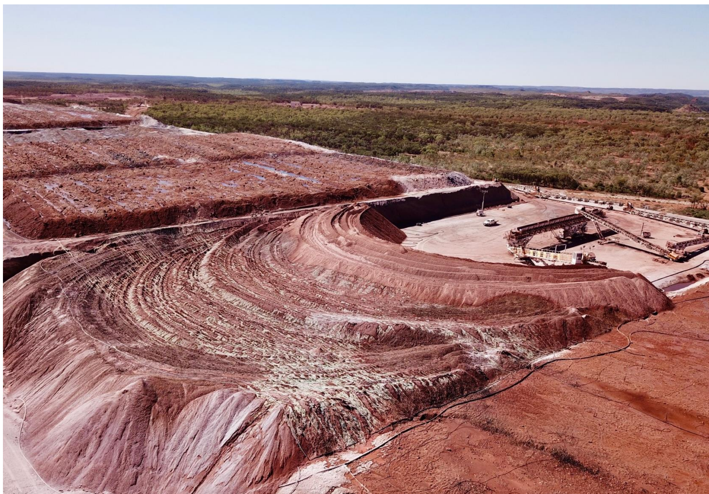
Figure 2. Stacker laying down Anthill ore on Pad 8. Over 70,000t stacked to date, representing the first 700t of recoverable Anthill copper cathode. Irrigation dripper lines to the left of the stacker, laying on surface. Leach solution percolates through heap and is collected by a network of drain pipes at base of heap. Copper levels in Pregnant Leach Solution commenced build-up within days of commencing irrigation.
