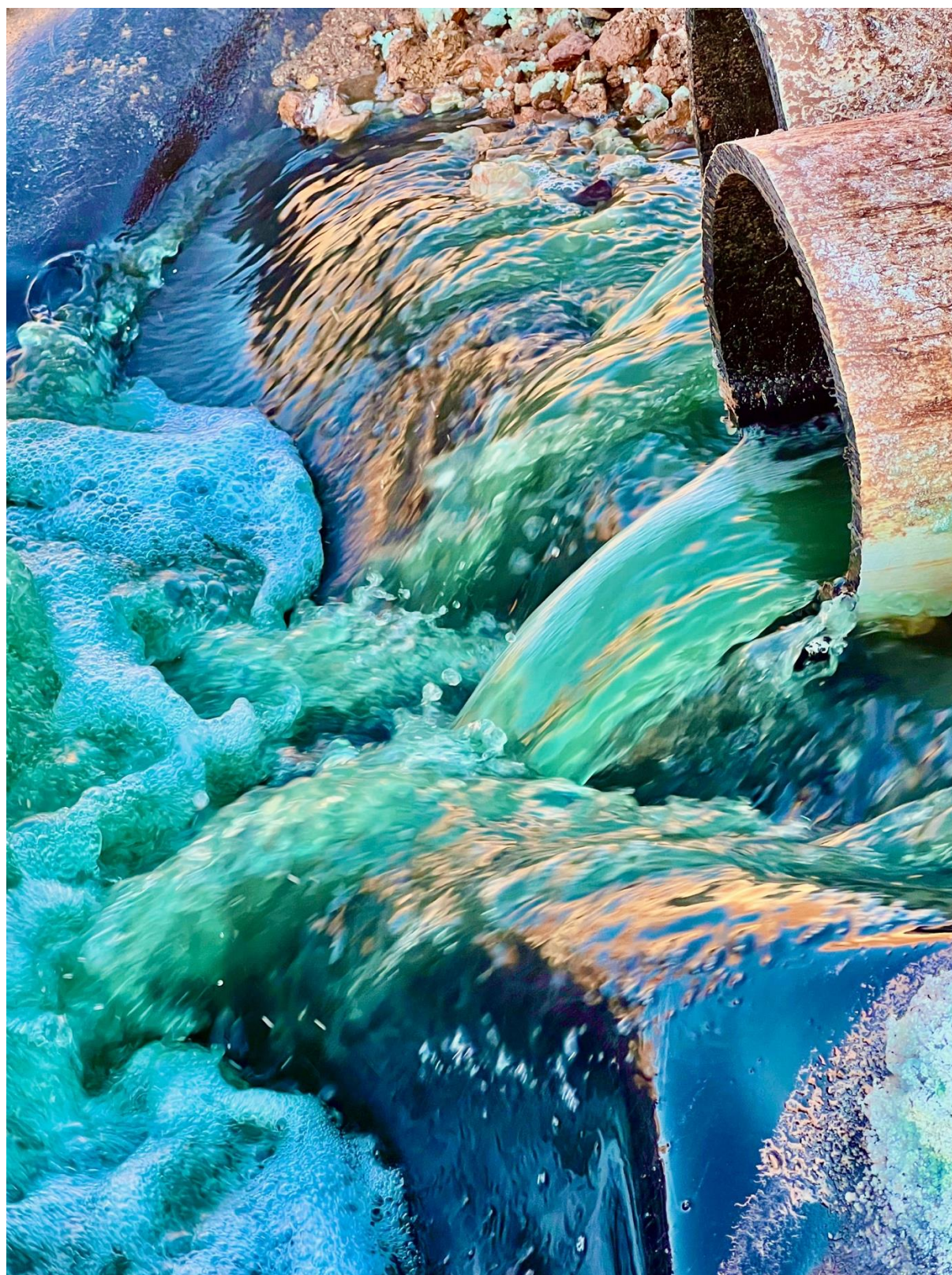
Figure 3. Copper-laden leach solution (green). This has percolated through the heap leach and is on its way to the PLS ponds for concentrating and electrowinning.
