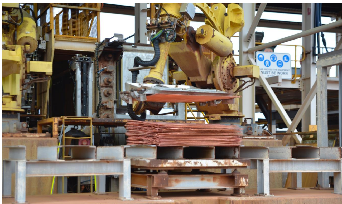
Figure 5. Robotic cathode stripping and stacking.
