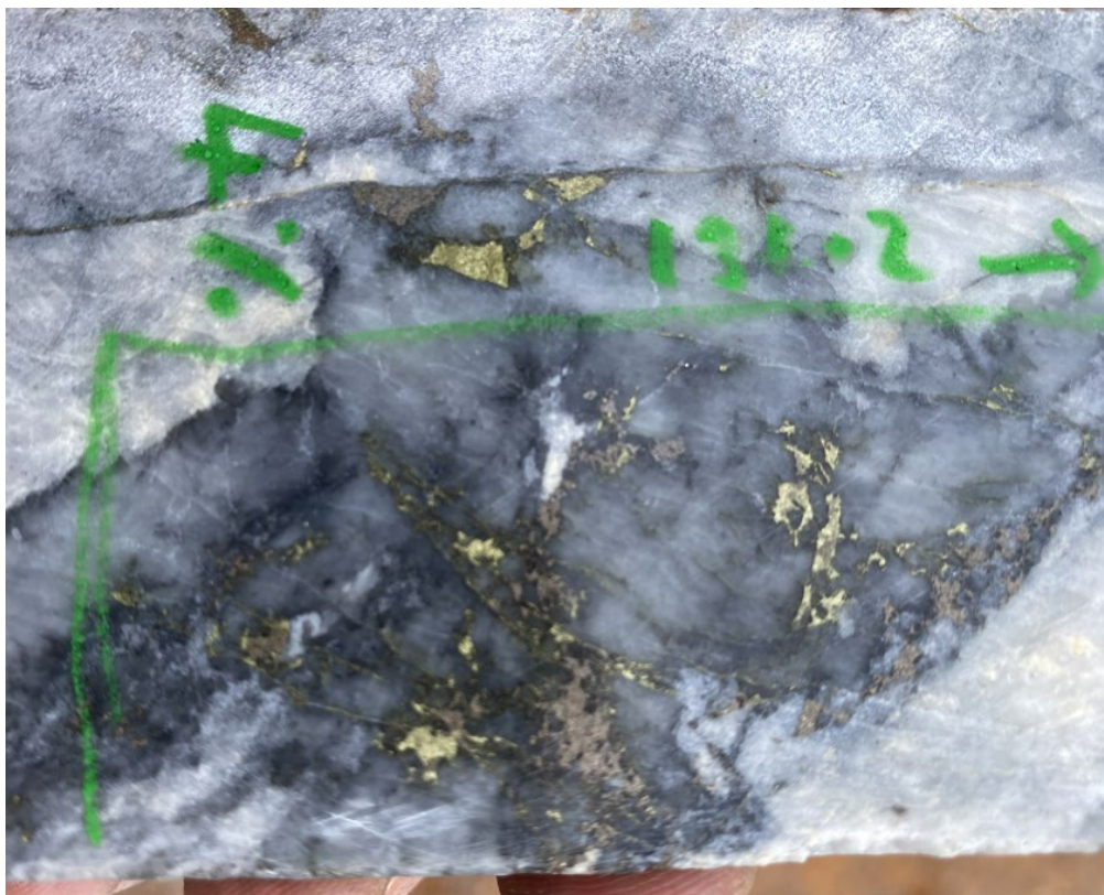
Figure 7 – LD22DD001 @ 131m ( 2.76 g/t Au and 0.98 % Cu ) – pyrrhotite and chalcopyrite in quartz – carbonate breccia, light brown pyrrhotite (po) with yellow chalcopyrite (cpy).
