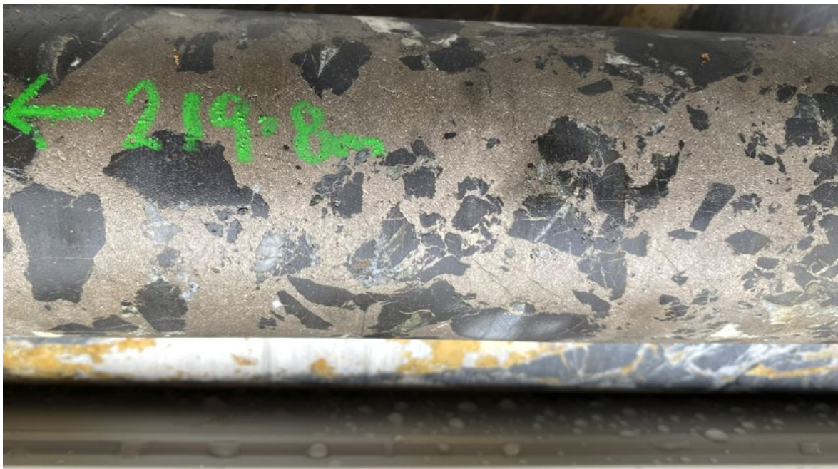
Figure 9 – LD22DD001 @ 219.8m – massive sulphides (pyrrhotite) in a shale breccia.
