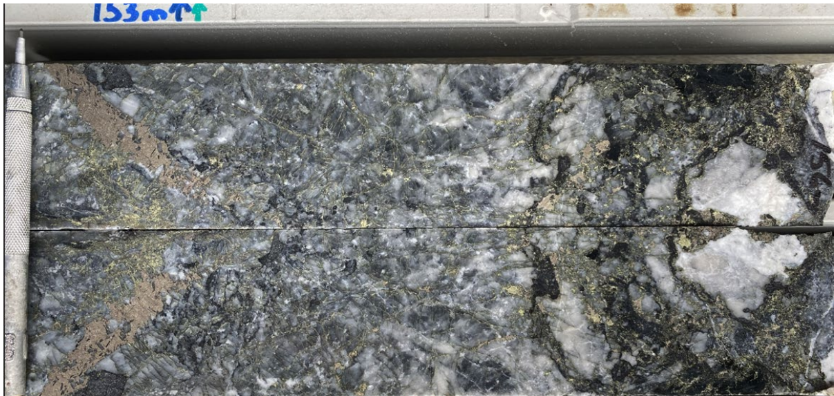
Figure 8 – LD22DD001 @ 154m ( 0.75 g/t Au and 1.08 % Cu ) – yellow chalcopyrite as stringers, veinlets and blebs; light brown pyrrhotite in a quartz-carbonate/ shale breccia.
