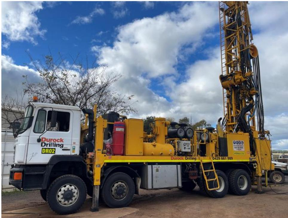
**Figure 1: Durock UDR 1000- with a 1150CFM /350psi compressor on board**
