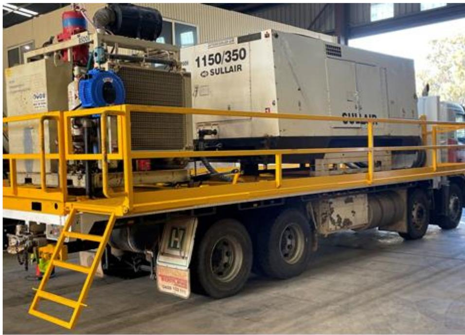
**Figure 2: Air truck with 1150CFM /350psi compressor (front)
