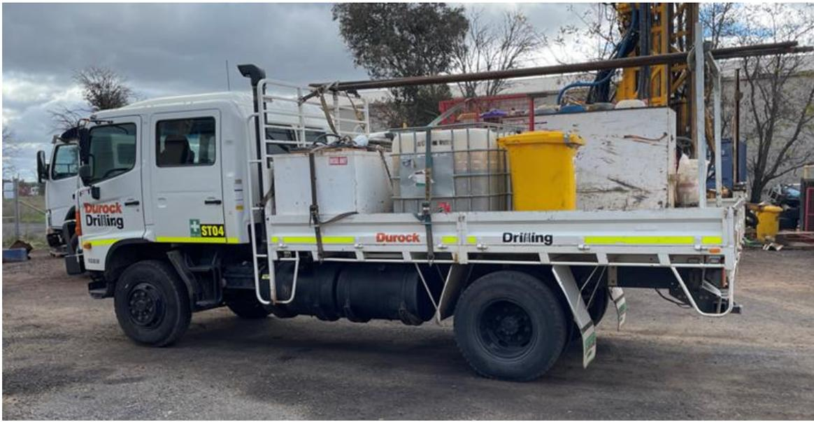
**Figure 3: Support Truck, 2,000L of diesel and 1,000L water**
