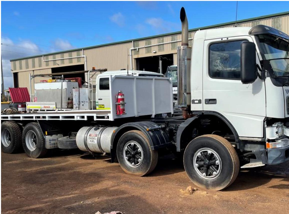
**Figure 4: Rod Truck, carries 400m of rods**
