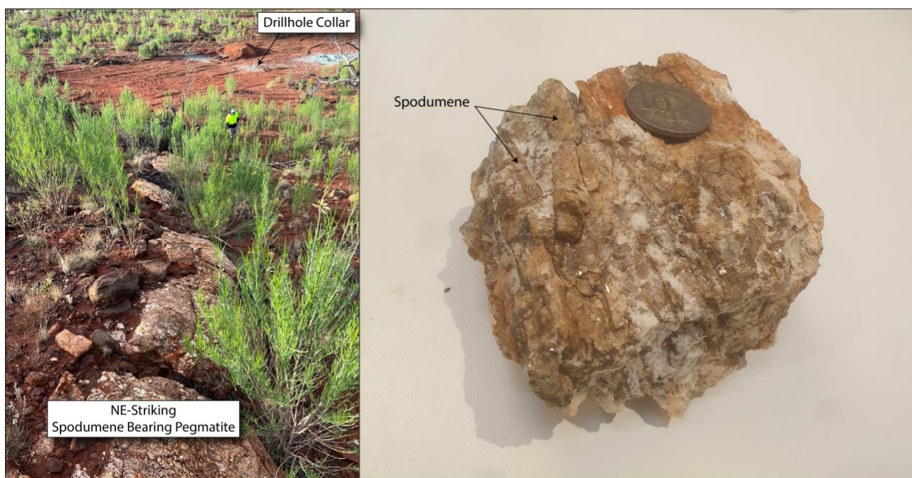
Figure 1: LEFT – Outcropping, spodumene bearing pegmatite. RIGHT – Grab sample collected from outcrop with abundant, elongate spodumene crystals.
