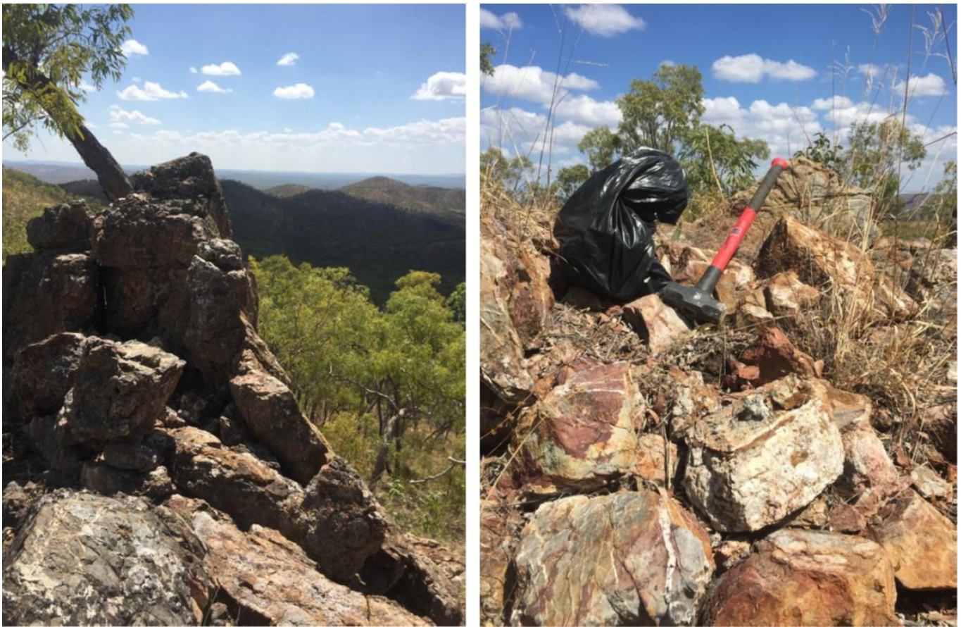
Figure 10. Bulk sampling of the oxidised Tornado quartz breccia vein for metallurgical test work by Gekko Systems.
