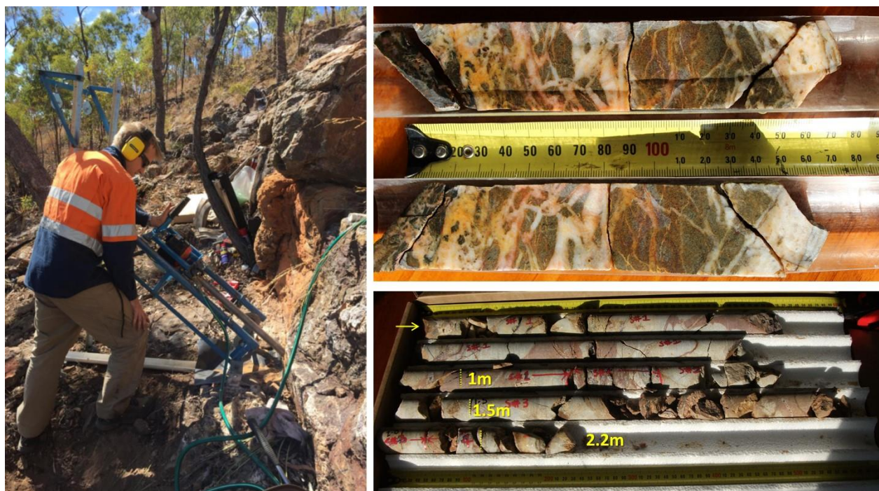
Figure 14. Diamond drilling of the Tornado quartz breccia vein by Placer Gold.
