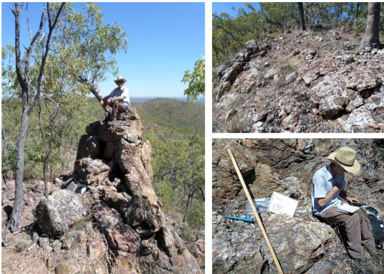
Figure 13. Rock chip sampling off the Tornado quartz breccia vein by Placer Gold.
