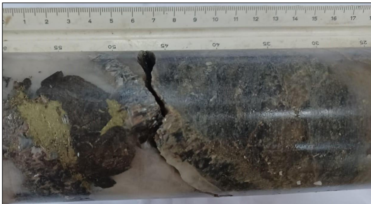
Figure 6. Milky quartz vein hosted in schistose metasediments with strong muscovite alteration and cassiterite-chalcopyrite mineralization. The photo is from ddh PN02, 288.60m and the scale is in cm.
