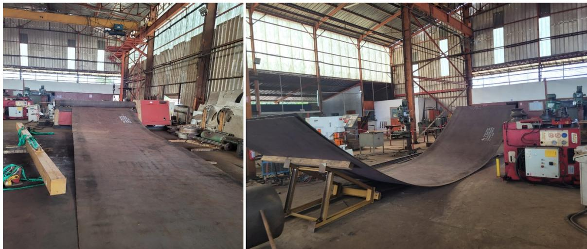
*Figure 8: Steel plates for CIL tanks being rolled in Abidjan workshop*
