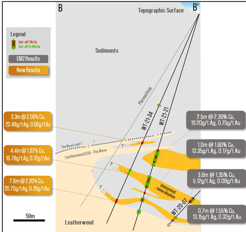
Figure 5 – East-west section through drill holes WT-21-34 showing location mineralised intersections and their spatial correlation with the Wave. See Figure 1 for section location. (Refer also announcements 29 October 2021 and 29 January 2021)
