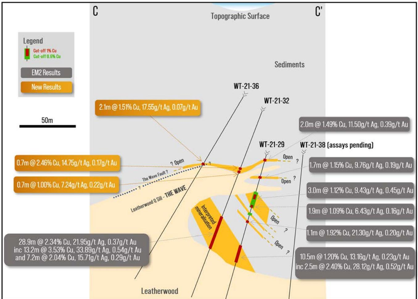
Figure 6 – East-west section through drill holes WT-21-36 showing location of mineralised intersections and their spatial correlation with the Wave. See Figure 1 for section location. (Refer also announcement 29 October 2021)
