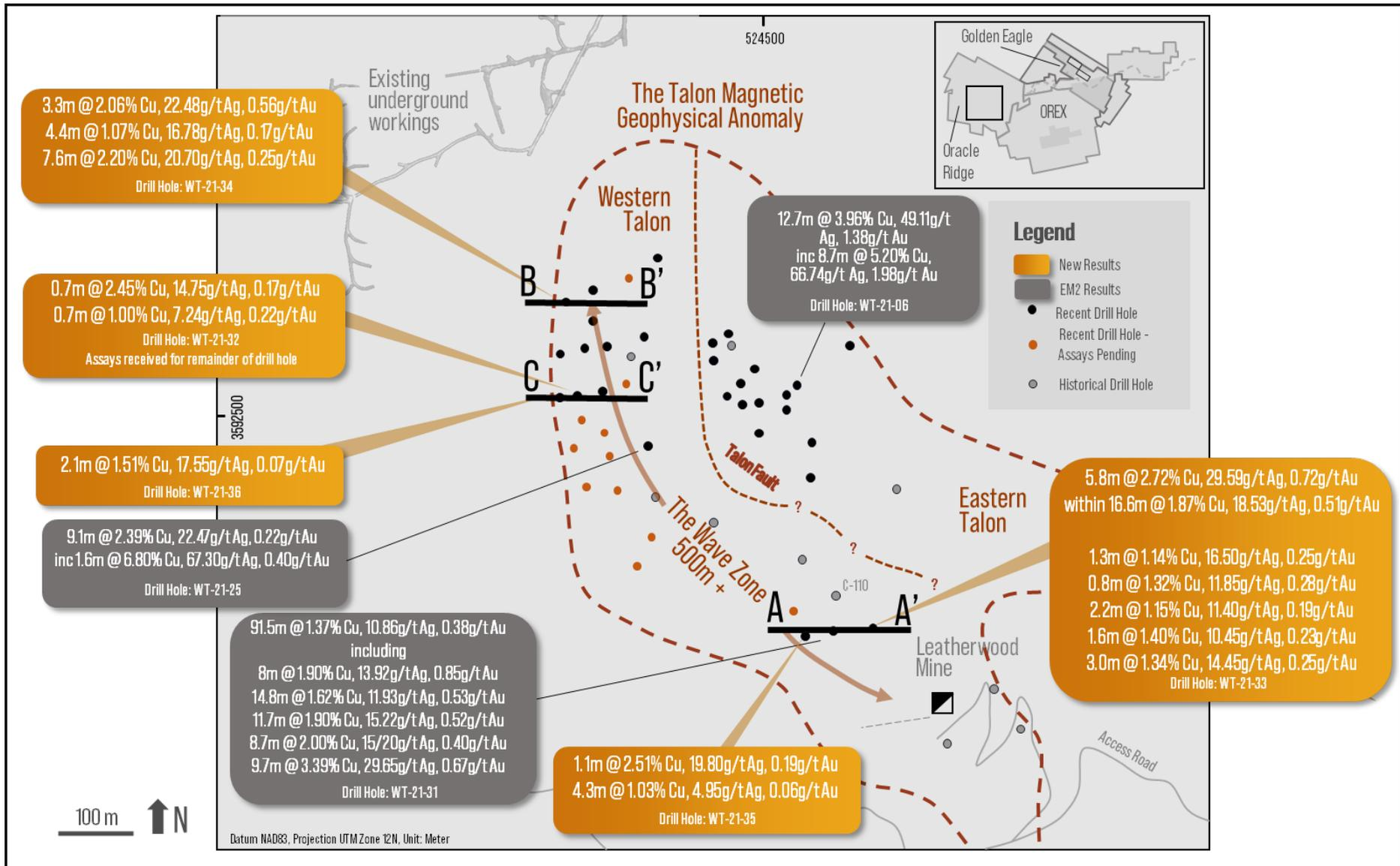
Figure 2 – Plan view of the Talon target showing reported results along the Wave zone. Due to the geometry of the drilling completed (e.g. fan drilling from a limited number of pads) the circles represent the approximate pierce point of each hole through the Leatherwood-Sediments contact. (Refer also announcement 29 October 2021)
