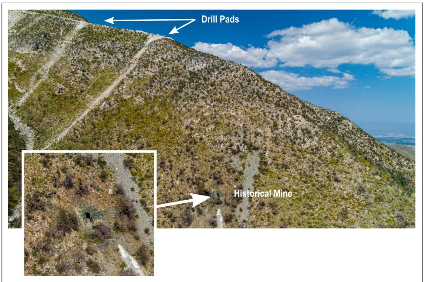
*Figure 3 – Surface photo of the southern end of the Talon area showing location of historical workings in the Leatherwood Mine area with recent drill pads higher on the ridge. Note the abundant green copper staining near the mine entrance.*
