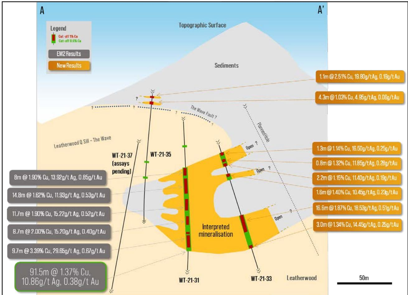
Figure 4 – East-west section through drill holes WT-21-33 and WT-21-35 showing location mineralised intersections and their spatial correlation with the Wave. See Figure 1 for section location. (Refer also announcement 29 October 2021)
