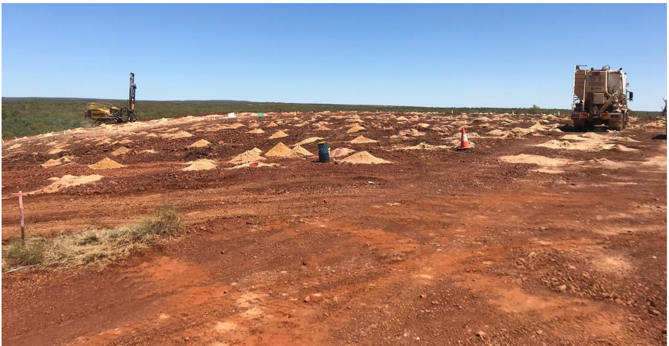
Figure 6. Blasthole drilling rig on left, emulsion truck on right.
