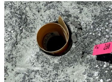
Fig 3. Collar Keeper profile in hole
