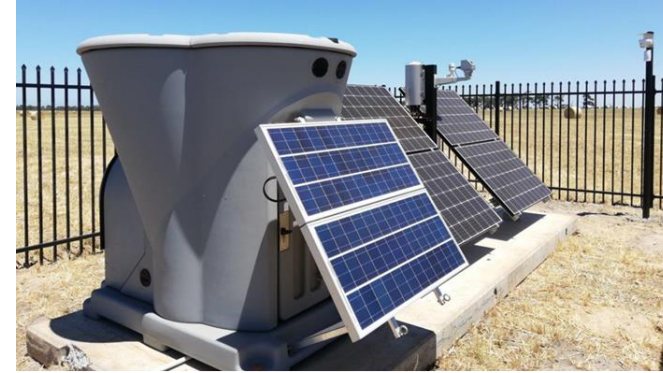
SODAR solar unit installed for 2022 Pre-Feasibility Study into the establishment of a Renewables Energy Hub
