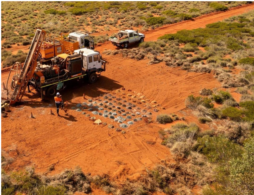
Figure 1: A drone aerial image of exploration drilling being undertaken at Roberts Hill.
