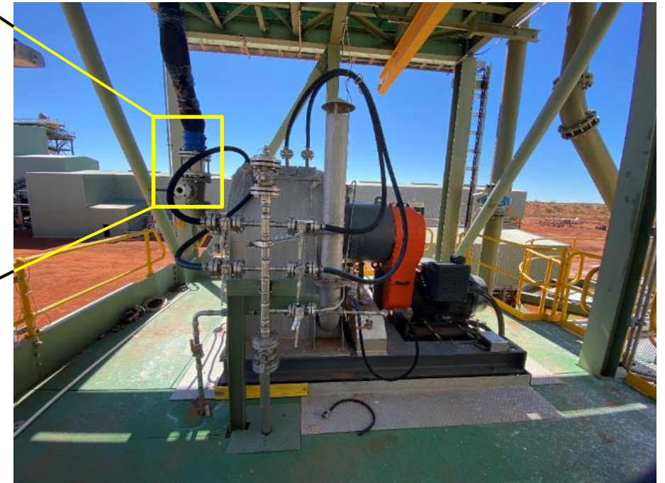
NaCl Centrifuge (Solid / Liquid Separation)
