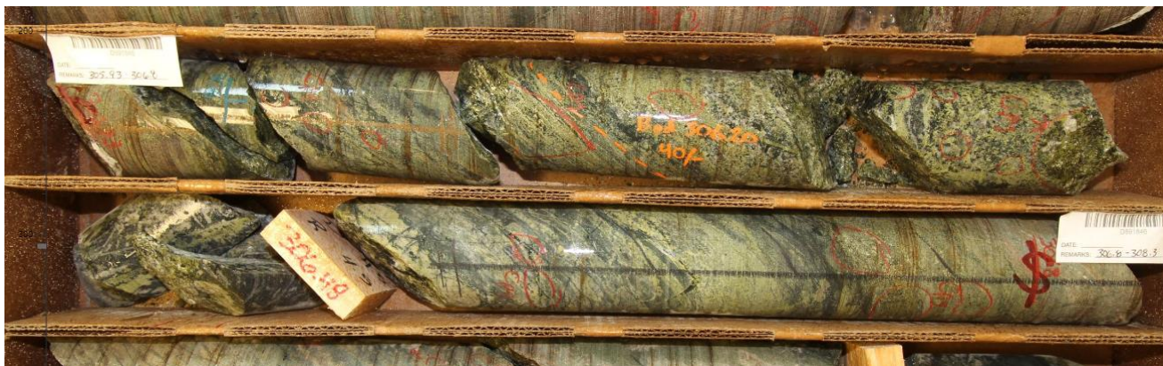
Figure 4 – Hole WT-21-39 at ~306.5m showing chalcopyrite mineralisation within skarn alteration. Mineralisation was within a 0.9m zone assaying 3.07% Cu, 12.50g/t Ag, 0.36g/t Au
