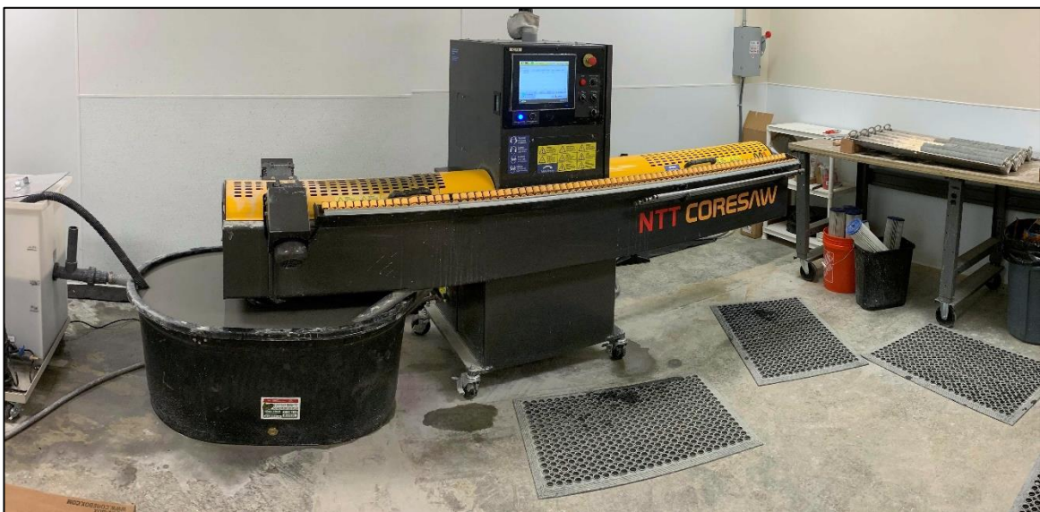
Figure 7 – Automatic core saw in operation at the Company's logging facility in Tucson, Arizona.
