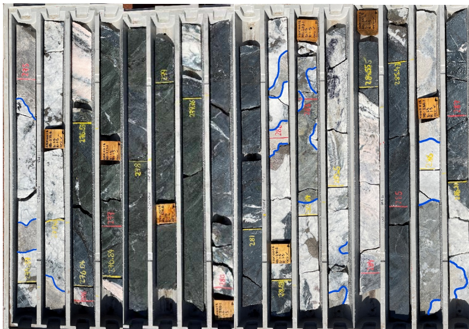
Photo 1: Cummins Range deepest intercept to date with patchy to massive monazite – outlines of the massive monazite in blue (note: monazite typically runs 60-70% TREO)
