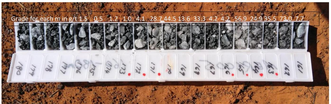
**Figure 3: Chip tray from MERC005 with 16m @ 20.92g/t high grade intercept from 161m**
