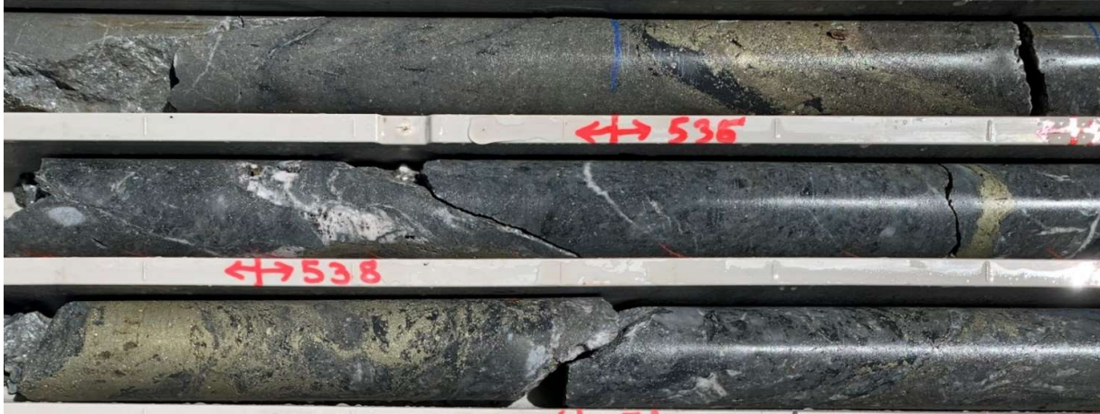
Figure 3: Detail of core with intervals of visible chalcopyrite and lesser pyrite, from first three rows of tray 10 in Figure 2 above that extend downhole from 46.2-48.7m (Diamond drill hole CRR21DD_011A, Scale: NQ core 50mm diameter variety)
