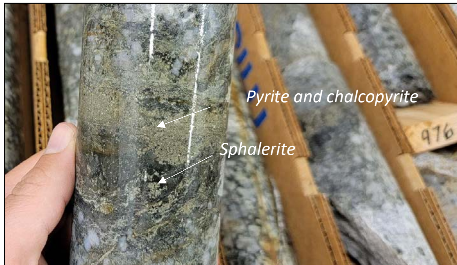
Figure 6 - Example of polymetallic veining seen in silica flooded, pyrite-rich alteration zone at Golden Eagle. GE-21-09 at 295m downhole depth. (refer ASX announcement 28 October 2021)
