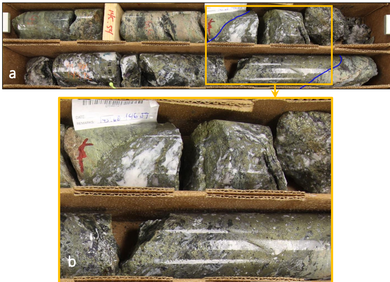
Figure 2 – a) High-grade quartz-calcite-chalcopyrite vein cross-cutting skarn-hosted mineralisation in drill hole WT-21-51 (145.4 to 146.5m downhole). Vein boundaries are shown in blue. b) Detail of image a) (orange inset) with abundant chalcopyrite in dark yellow-green colour.
