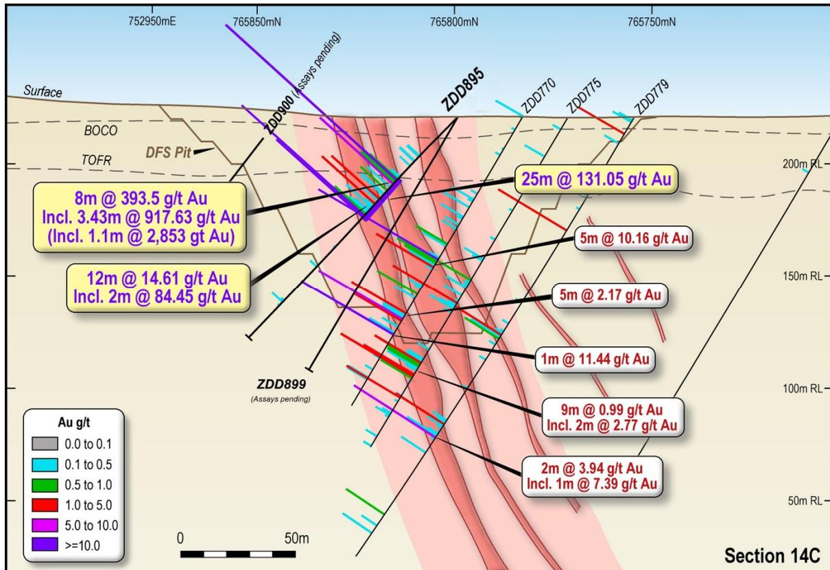
Figure 5: Oblique cross section showing latest drill results at AG Core (section 14C +/-12.5m)
