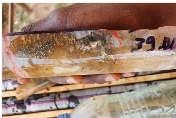
*Figure 1: Diamond drill core from interval 38.57m - 39.67m in hole ZDD895 at AG Core (NTW core diameter of 56.1mm)*
