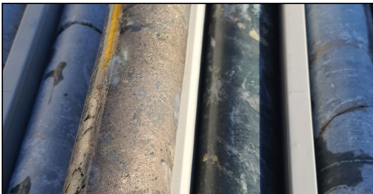
Figure 4. Semi massive and disseminated sulphide intersected by NDD0010 around 140m downhole. The hole size is NQ2.
