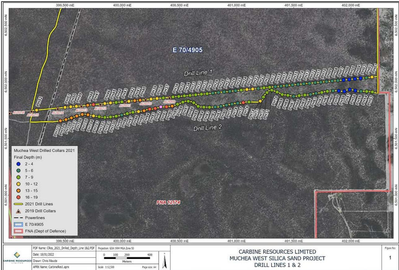
**Figure 4: Drill spacings and hole depths Lines 1 and 2**
