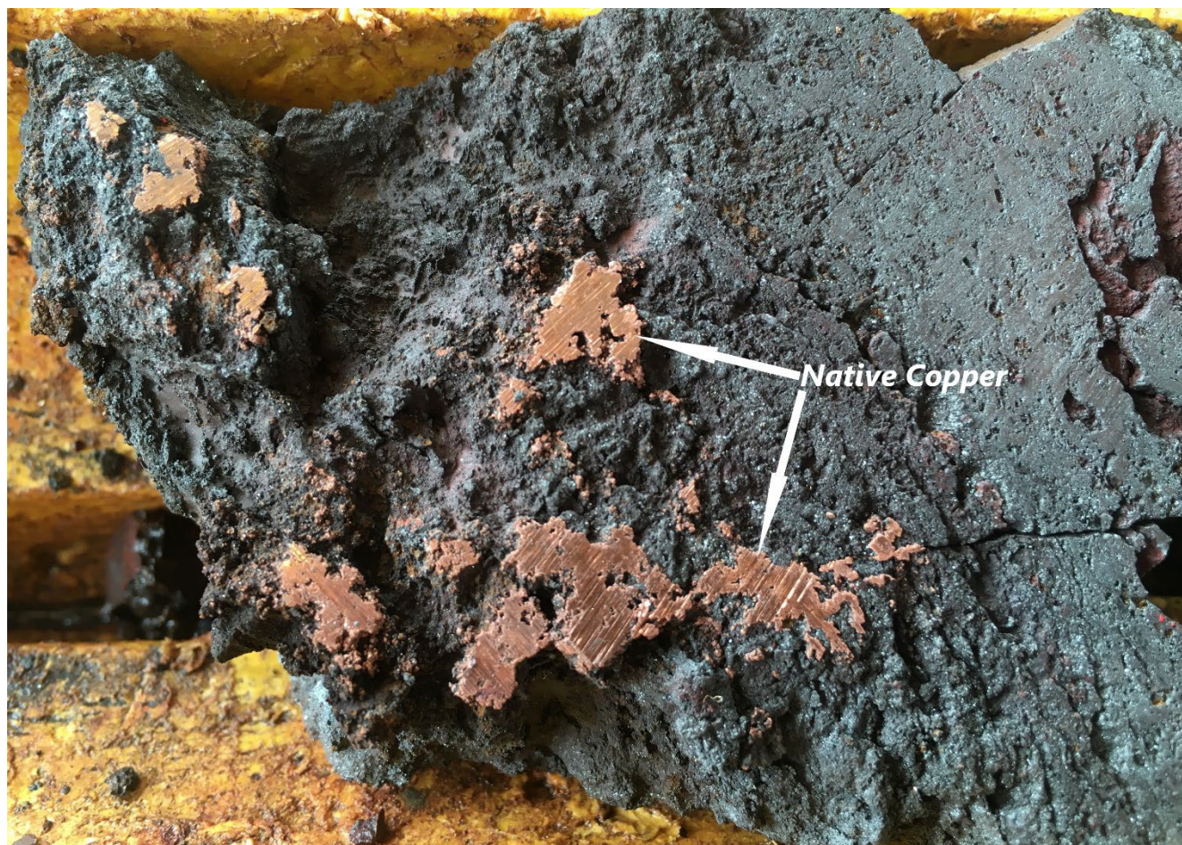
Photo 1: Native copper in ironstone/haematite altered cut HQ sized drill core, BBDD0011, 206.5m down hole
