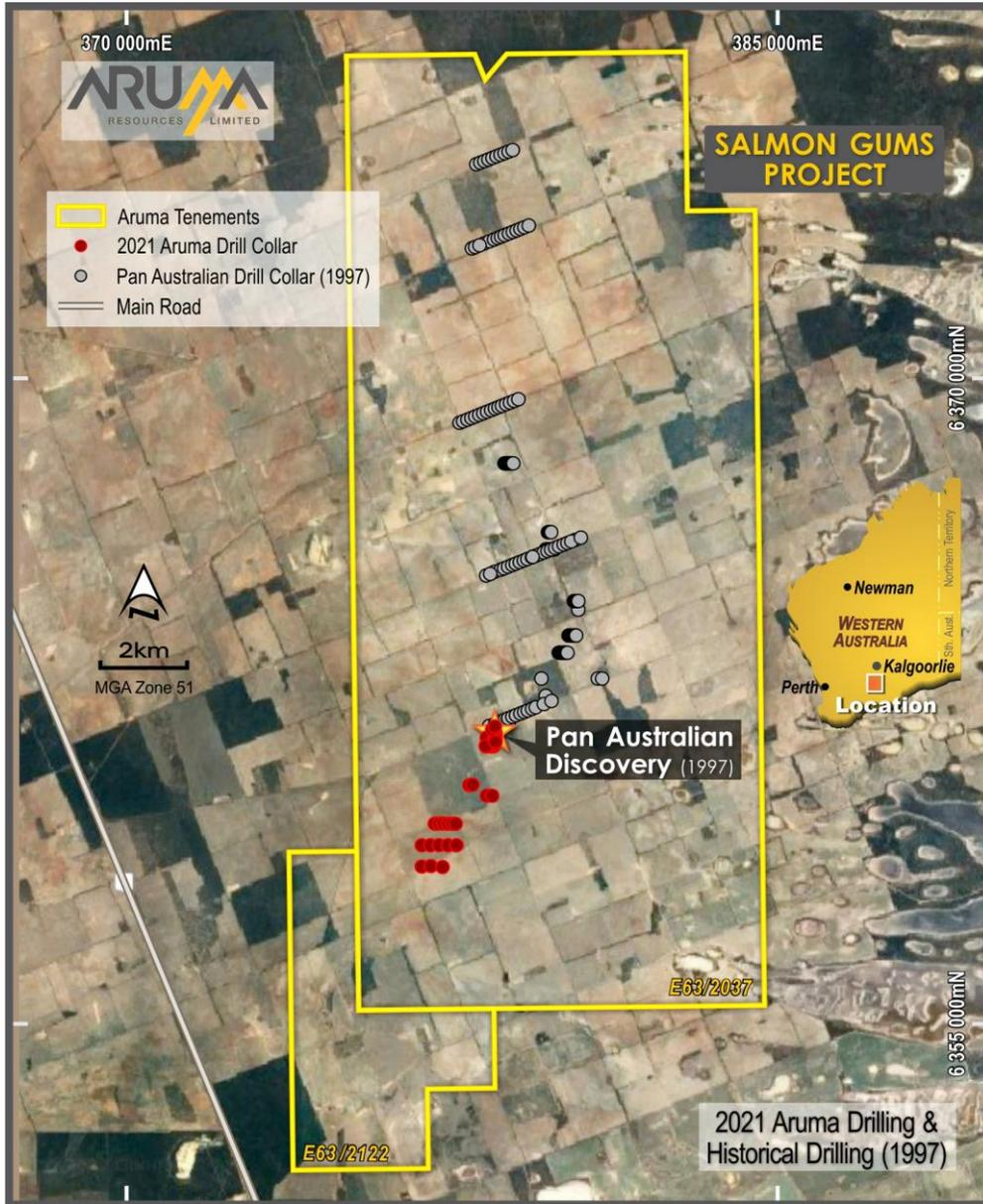
**Figure 1:** Drilling location Plan for Salmon Gums showing the November Drilling which is detailed in Figure 2 below
