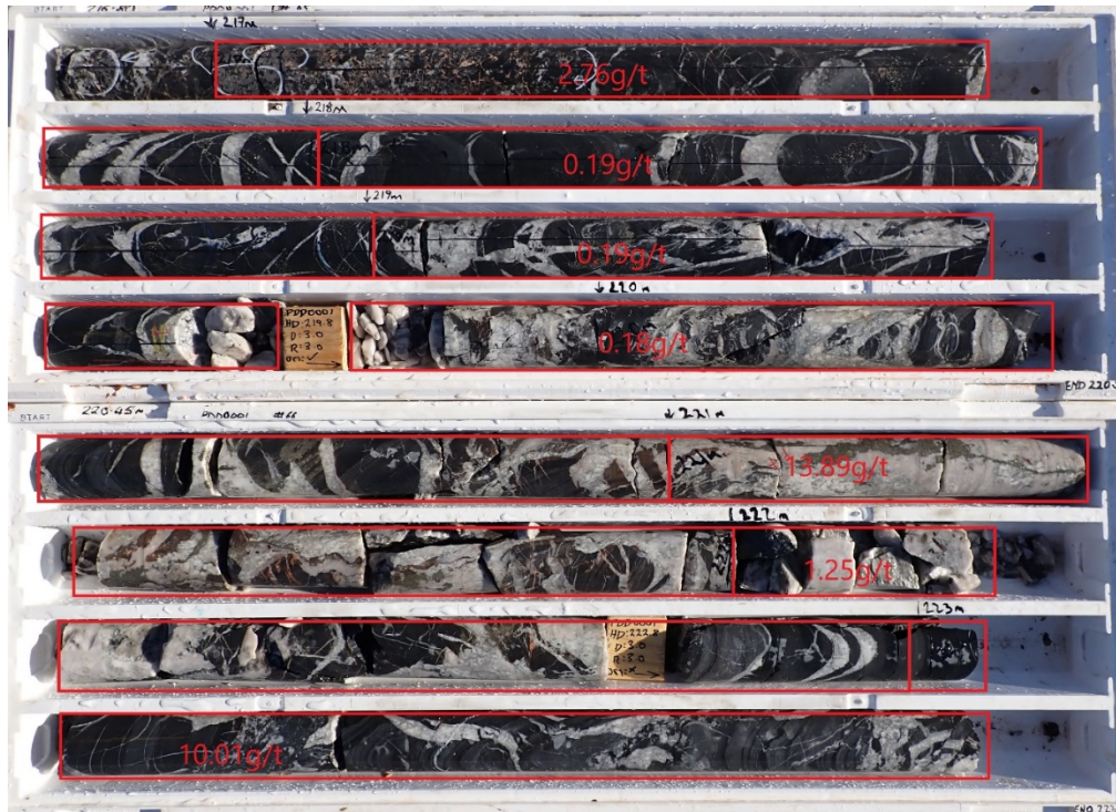
Figure 2: Silicic-carbonate veining and alteration in PDD0001 with pervasive sulphidation. Gold grades noted over the intervals from 216m to 224m.
