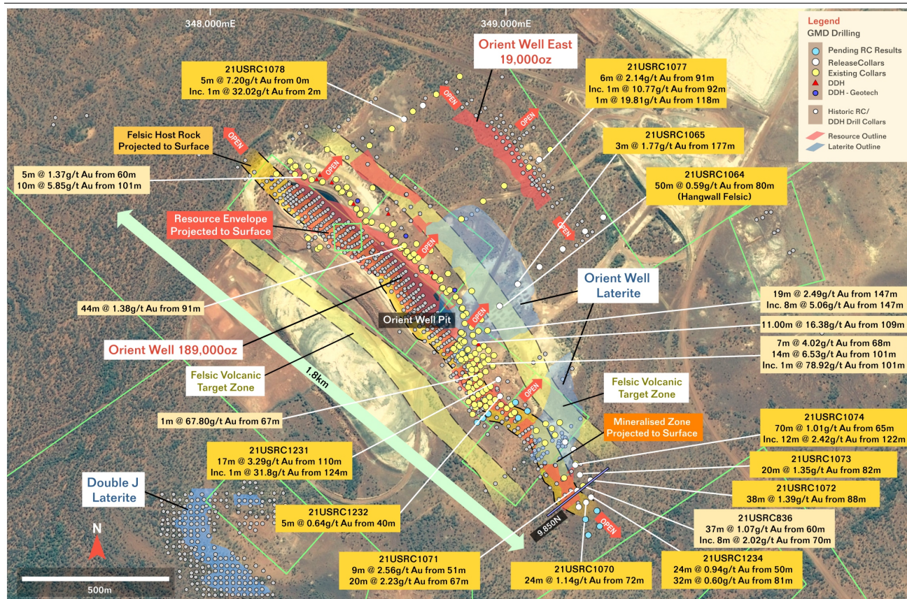
Figure 8. Orient Well extensional drilling shown in plan view. Recent drilling intercepts shown in yellow boxes and previously reported Genesis drilling in light yellow boxes. Drill hole collar locations highlighted by white circles and the position of Figure 9 cross section highlighted.
