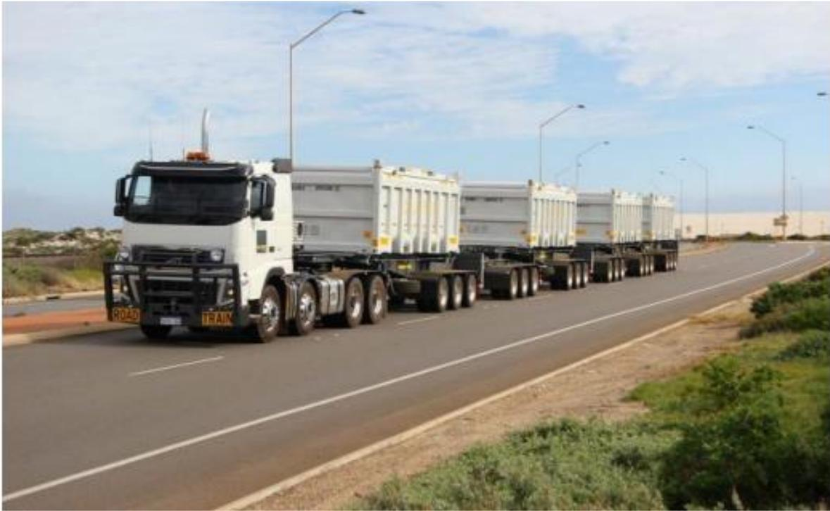
Figure 15: Indicative Quad Road Train Loaded with Rota-boxes
