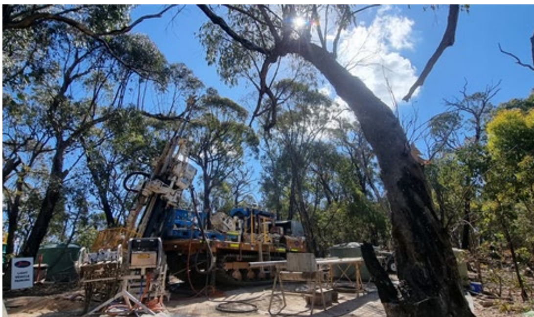
Figure 1: Deepcore drill rig in operation on hole MD16 at Malmsbury (Belltopper Hill). This hole is testing the Leven Star Reef.
