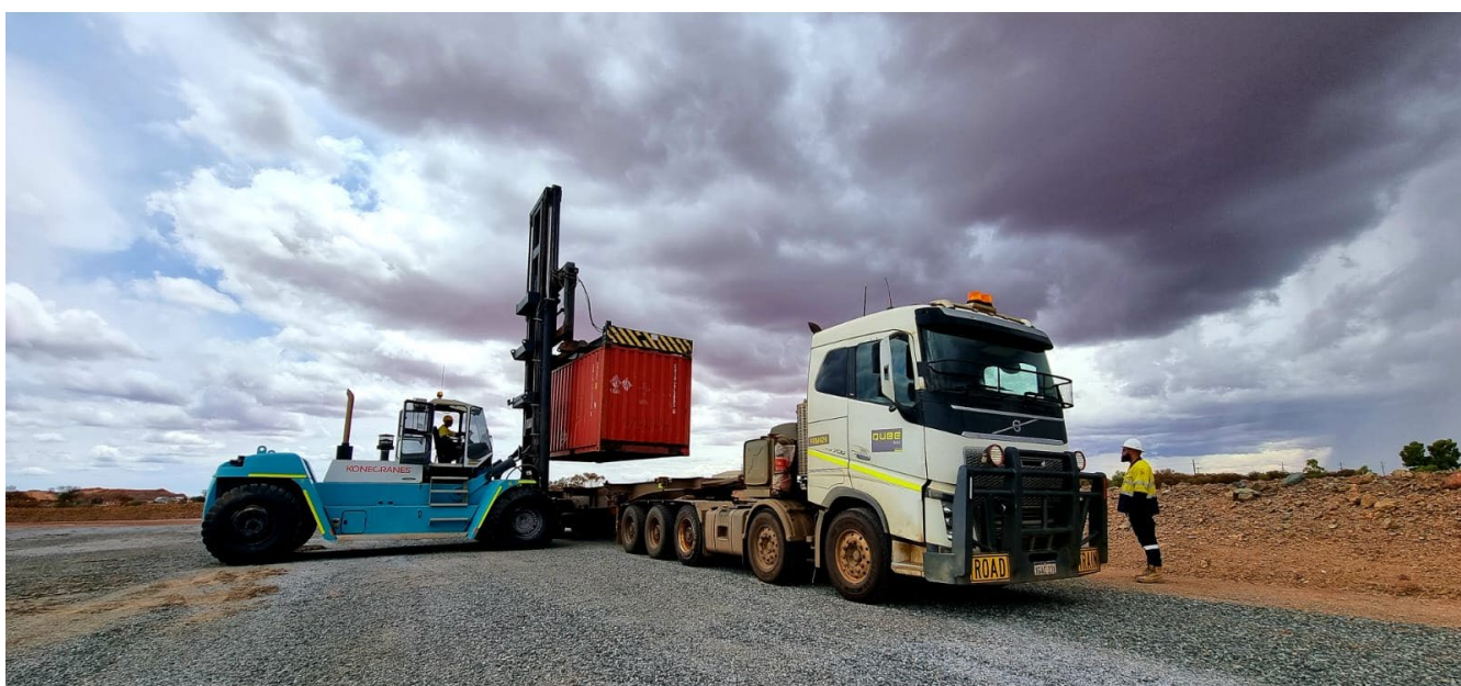
Figure 2 – containers of concentrate being loaded onto road train for transport to railhead
