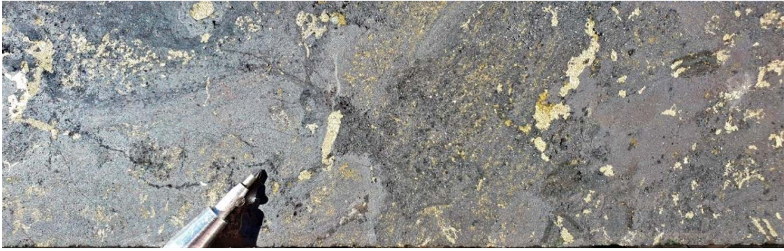
Plate 1a: VUD0019 - 1411.2m. Disseminated chalcopyrite and pyrite mineralisation in hematitic breccia. NQ2 ½ core.
