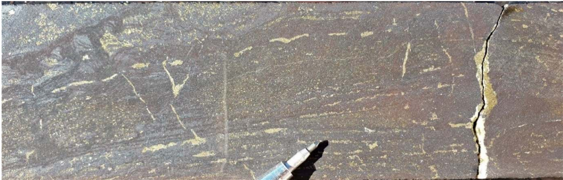
Plate 1b: VUD0019 - 1415.5m. Finely layered chalcopyrite and minor pyrite mineralisation in hematite breccia. NQ2 ½ core.
