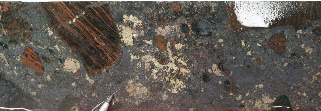
Plate 1d: VUD0019 - 1452.5m. Disseminated and blebby pyrite and lesser chalcopyrite mineralisation in hematite-rich polymictic breccia. NQ2 ½ core.
