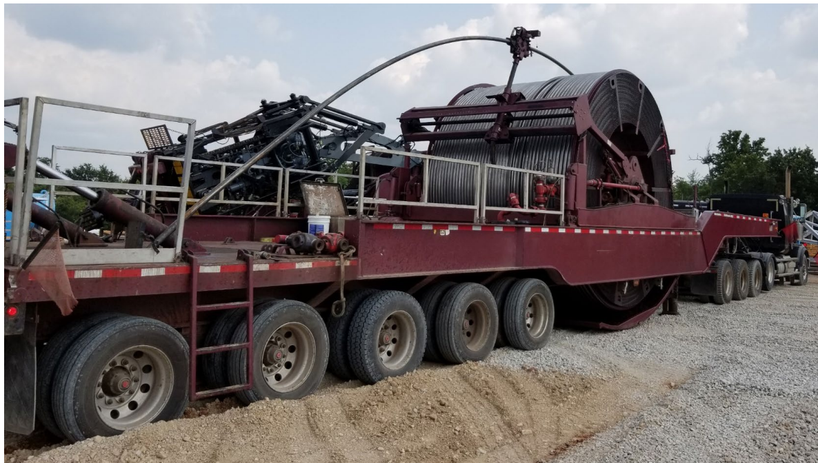
Figure 2: Rigging up coil tubing unit on the Jewell Well location in Carter County, Oklahoma
