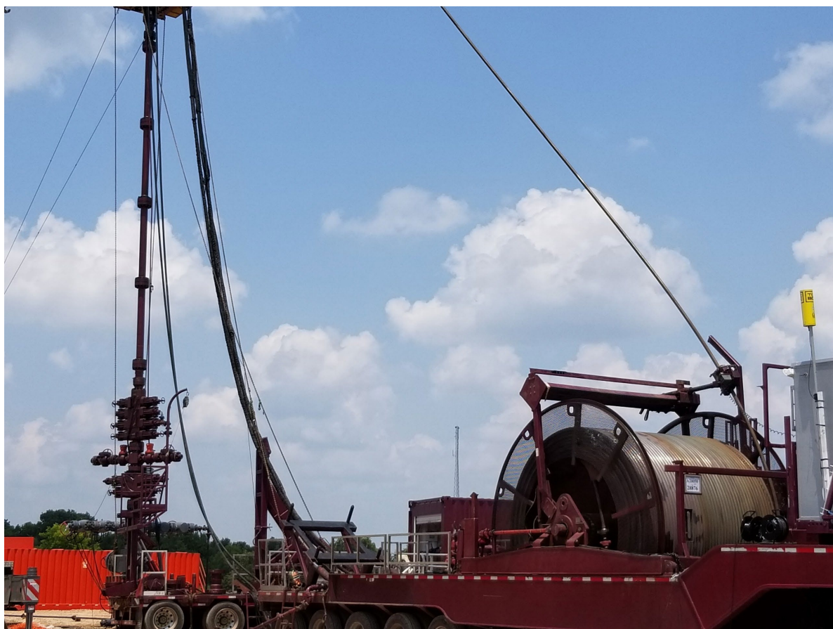
Figure 3: Entering the wellbore with coiled tubing, Jewell Well location in Carter County, Oklahoma
