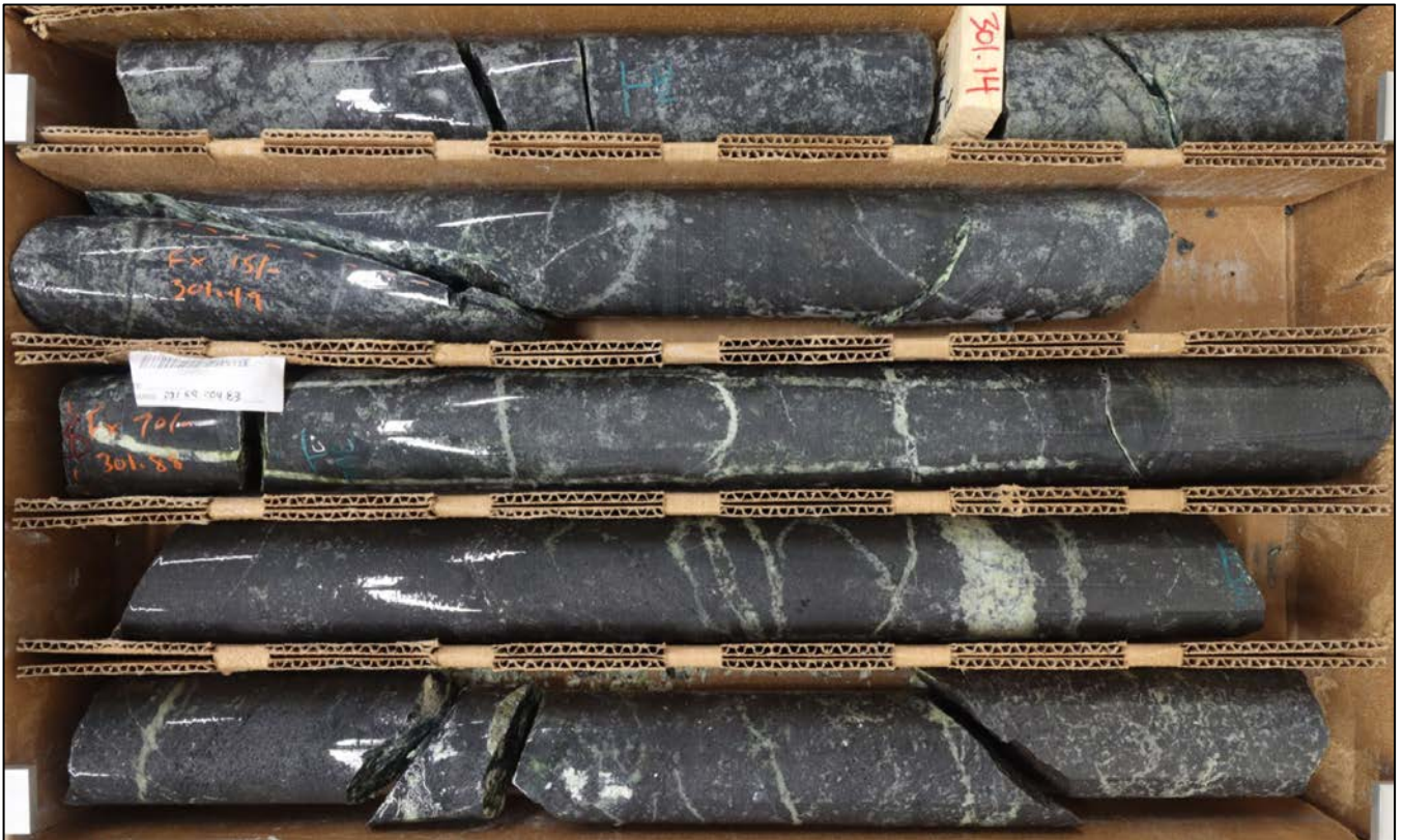
Figure 4 – Massive to semi-massive magnetite-sulphide interval in drill hole WT-21-22 (300.8m - 303.6m). Some of the best results to date in the eastern Talon area have been returned from similar mineralisation at the Leatherwood sediment contact.
