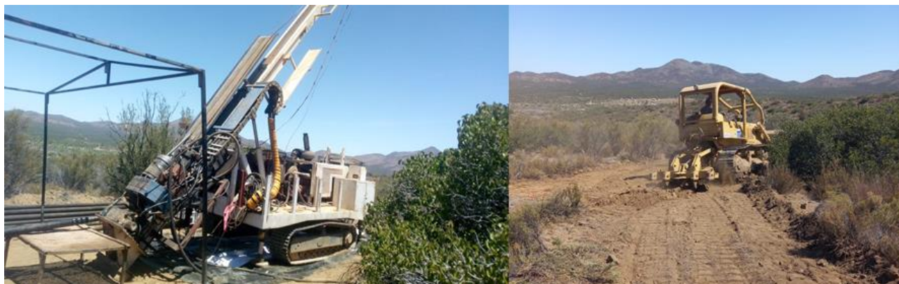
Figure 1: Track mounted drill rig positioned ready to commence drilling and Dozer clearing access tracks and drill pads for drilling.
