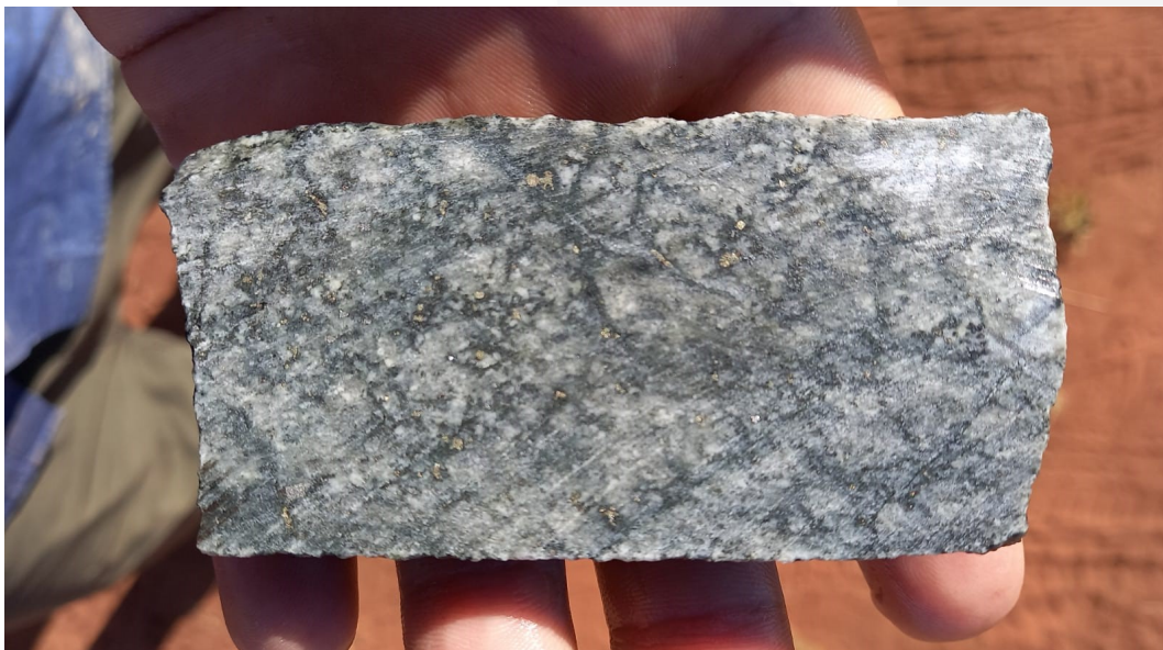
Figure 8. Bastion Prospect drill core photo from PLDD0005, 174.4m, 1.1 g/t gold hosted by disseminated sulphides in an intrusion.
