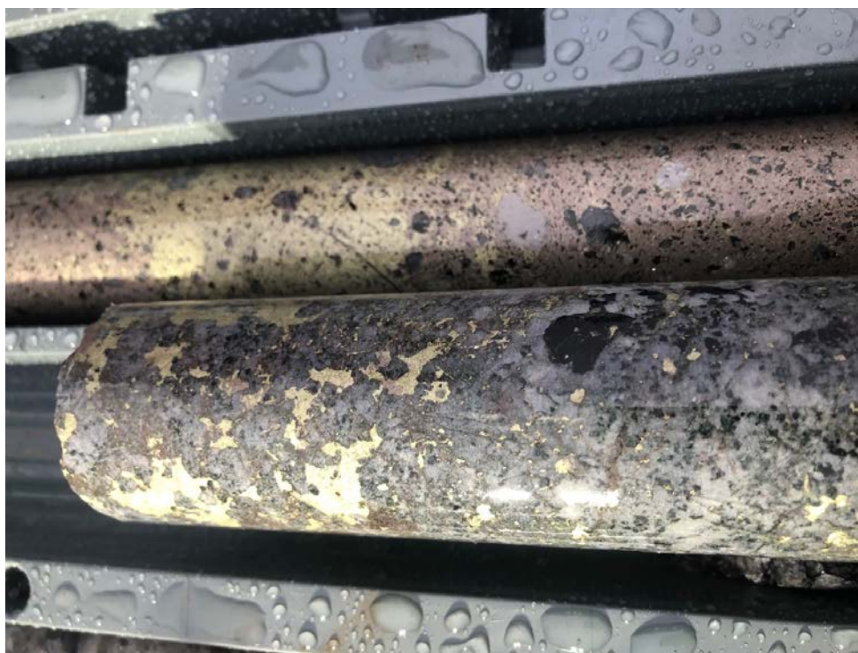
Figure 7 - 21PHDD002 Coarse-grained disseminated chalcopyrite and pyrrhotite in foreground and massive chalcopyrite and pyrrhotite with lesser arsenopyrite in the background.
