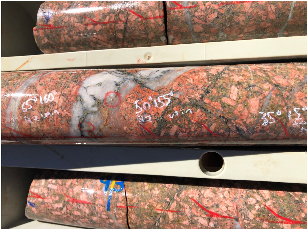
Figure 5 - HQ diamond core from BCDD2101 containing quartz veining with sulphide and visible gold in altered monzonite at 92m downhole
