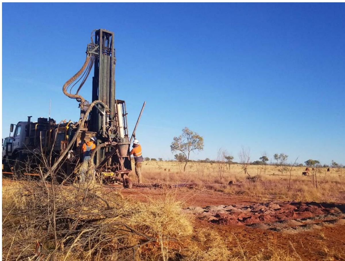
Figure 6 - Aircore drilling underway at PHD gold target July 2021
