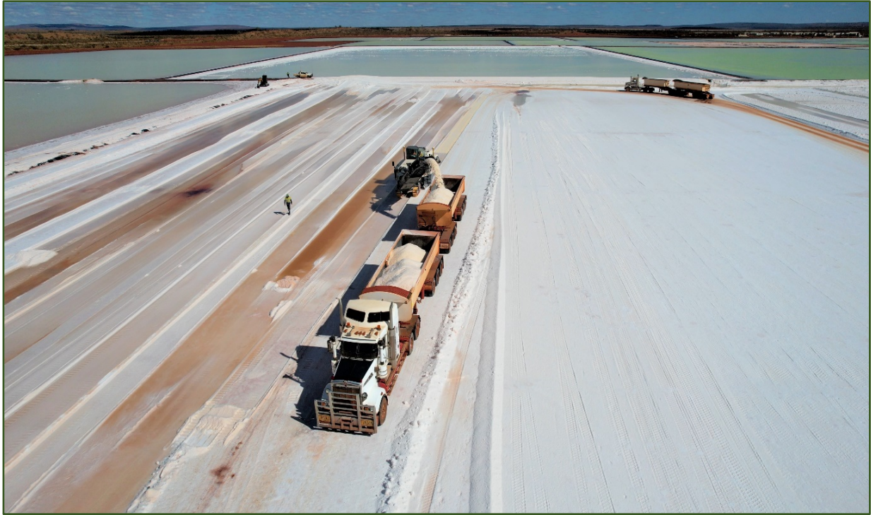
Salt Harvesting and Transport to ROM pad
