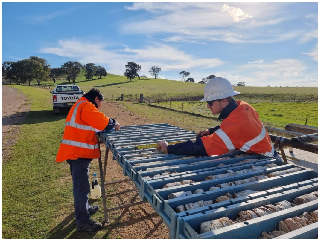
Figure 1 – Core logging at the Highway Prospect
