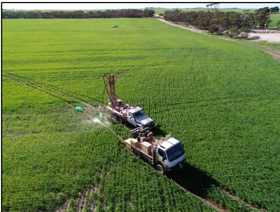
Figure 1: Air-core infill drilling at the Cloud Nine Deposit, Merredin WA
