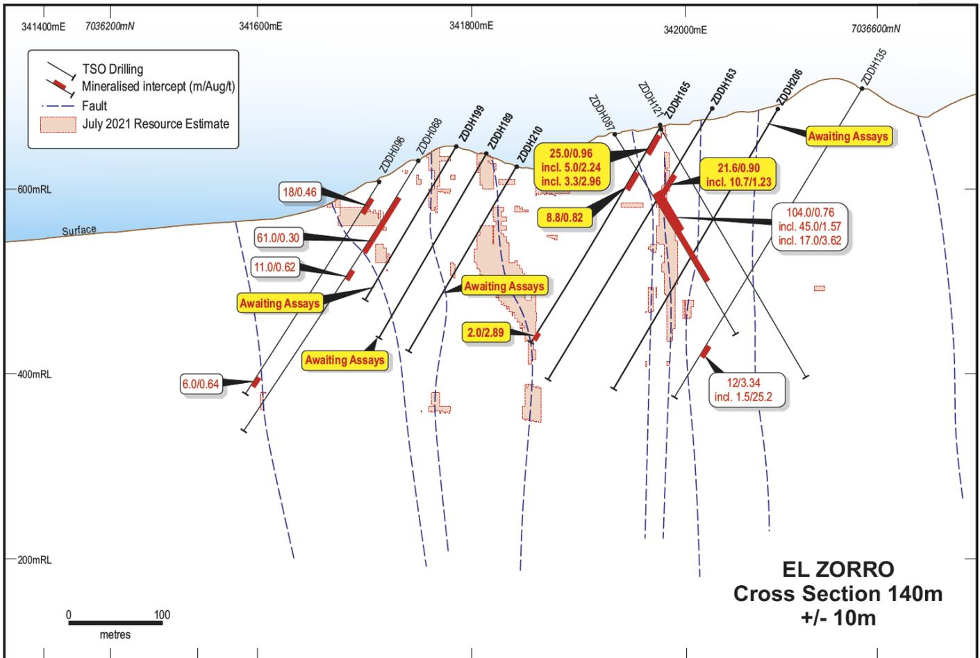
Figure 8: Ternerera Drill Section +140m looking northwest.
