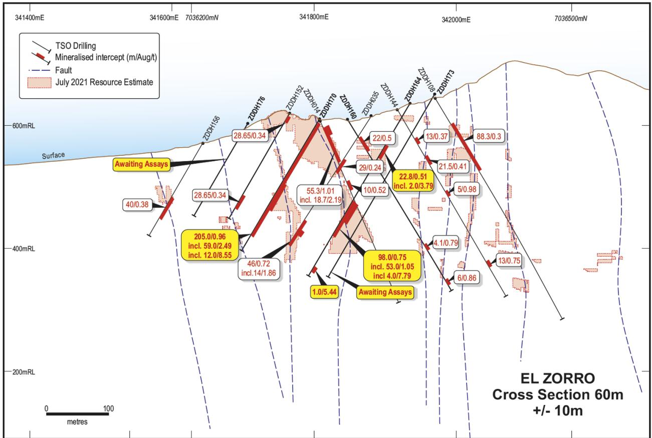
Figure 1: Ternera Drill Section +60m looking northwest. Hole ZDDH0170and ZDDH0164 showing strong gold mineralisation outside of existing Mineral Resource model and significantly expanding known gold zones.
