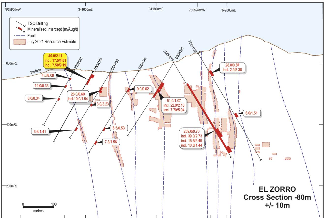
Figure 2: Ternera Drill Section -80m looking northwest. Hole ZDDH0168 showing gold mineralisation in the new western zone of Ternea outside of the existing Mineral Resource Estimate.
