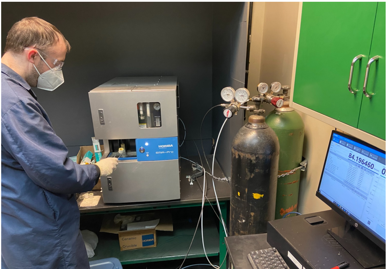
Sulphur analysed by infrared absorption method
