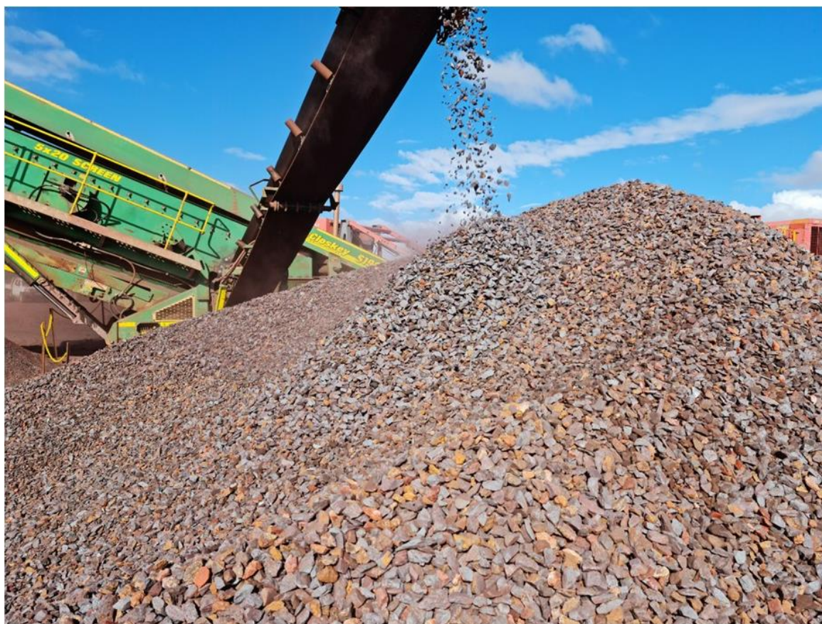
Figure 1 - Crushed material on the product pad ready for haulage to port
