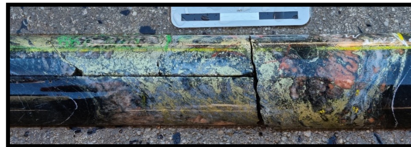
KSDD031 – 0.3m grading 43.4g/t Au, 7.8% Cu from 886.4m – Chalcopyrite-calcite-kspars altered monzonite finger within the breccia
