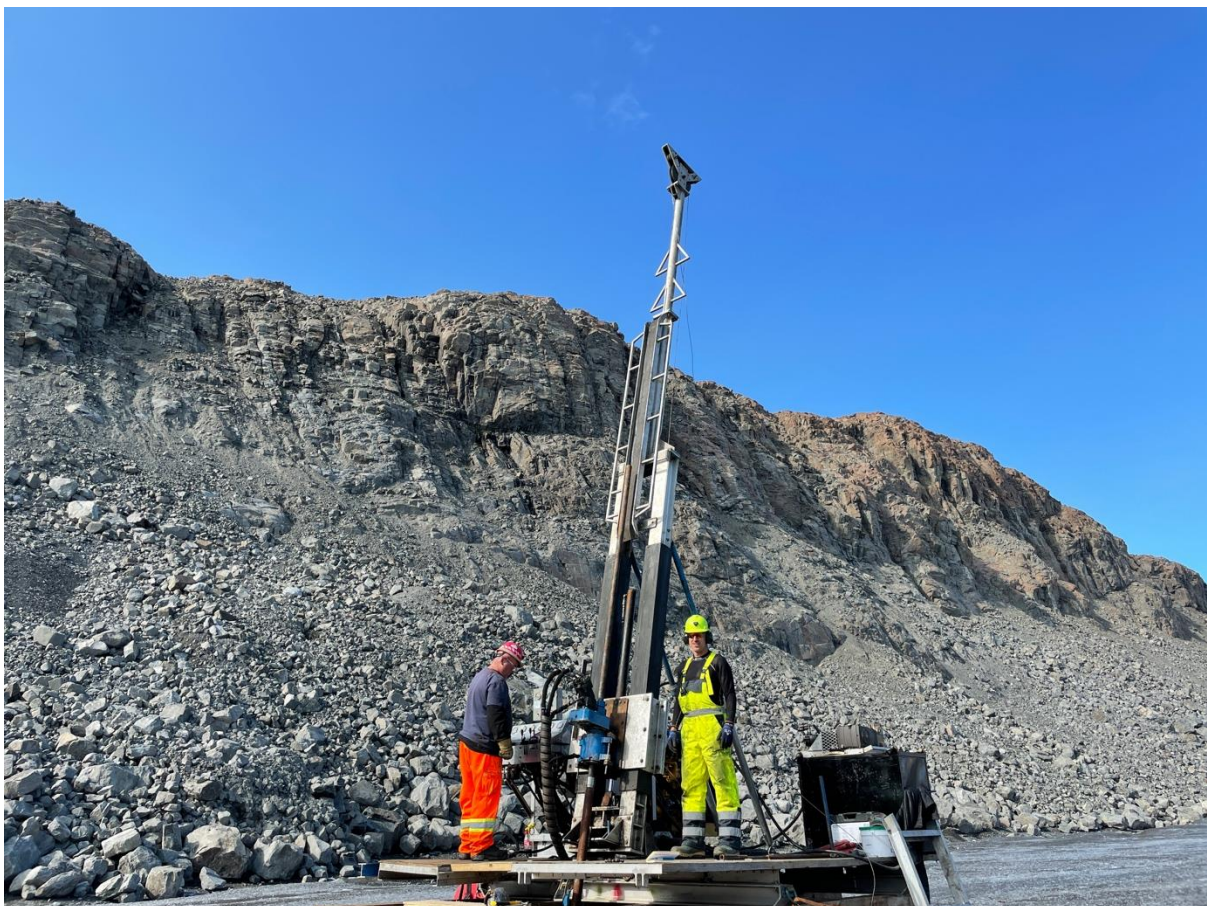
Figure 1 Diamond drill rig commencing coring at the Miki magmatic sulphide prospect on the 19 th July 2021.
