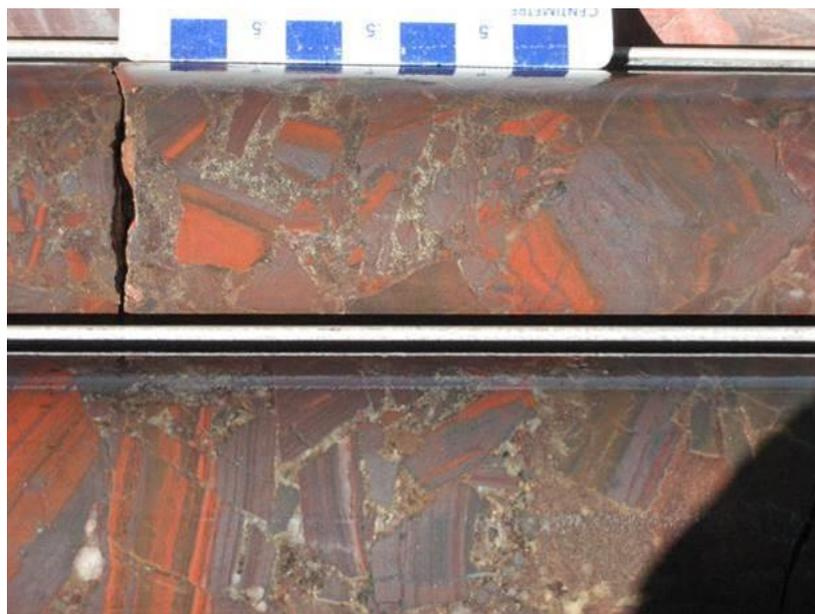
**Figure 15: Hematite-rich jaspilitic BIF from MPD001 below 1,288m**
