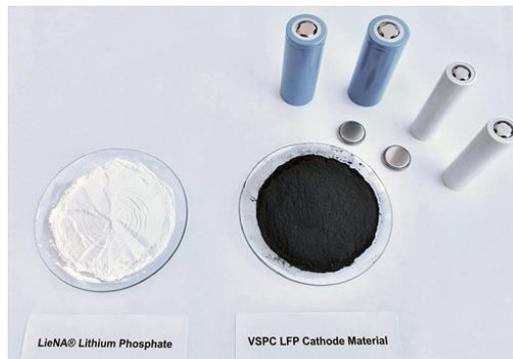
*LFP cathode material sourced from LieNA<sup>®</sup>-produced LP.*
