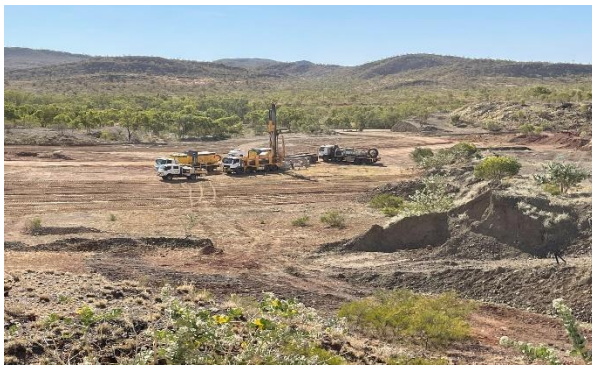
Image 5. Dewatering bore drilling in progress at Mt Freda.
