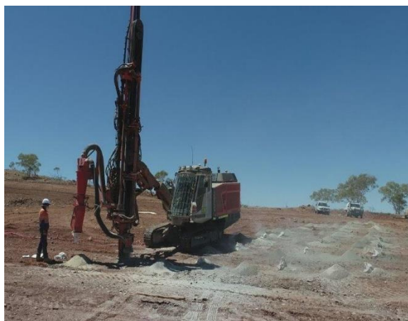
Image 2. First of the blast rigs has arrived on site and has commenced drilling.
