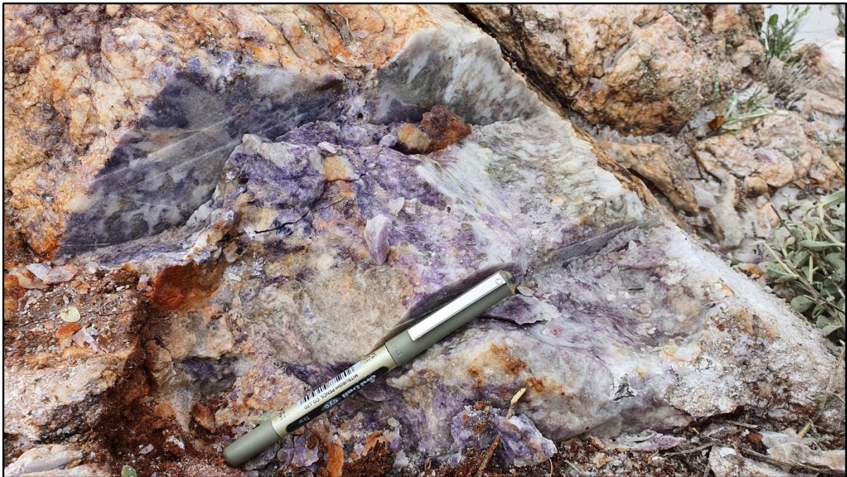
Figure 1. High-grade rubidium and lithium lepidolite pegmatite sample from Wyemandoo.
